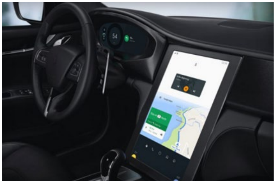
Android N OS running on screens (of head unit and instrument cluster) inside Maserati Ghibli (Source: Google)
